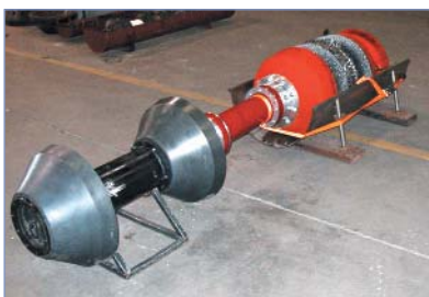
Figure 2. 20 and 24 in. coupling systems for a Magpie metal loss tool and a TDW caliper tool were recently designed to inspect a crude oil line in a single run.
